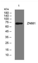
Western blot analysis of lysates from THP-1 cells, primary antibody was diluted at 1:1000, 4° over night
